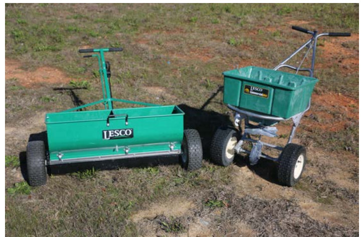
A drop spreader (left) and rotary spreader (right). Cory Tanner, ©2018, Clemson University
