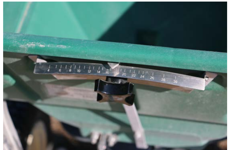
The spreader adjustment is set to the middle setting. Cory Tanner, ©2018, Clemson University
