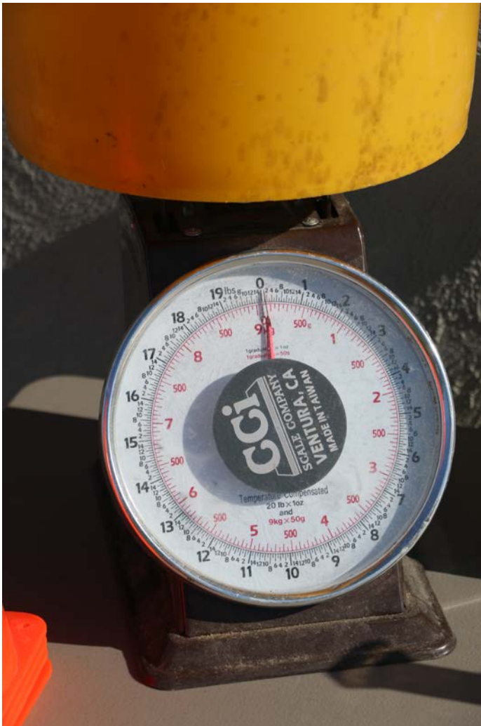
This scale has been tared for the weight of the bucket and now reads "0".
