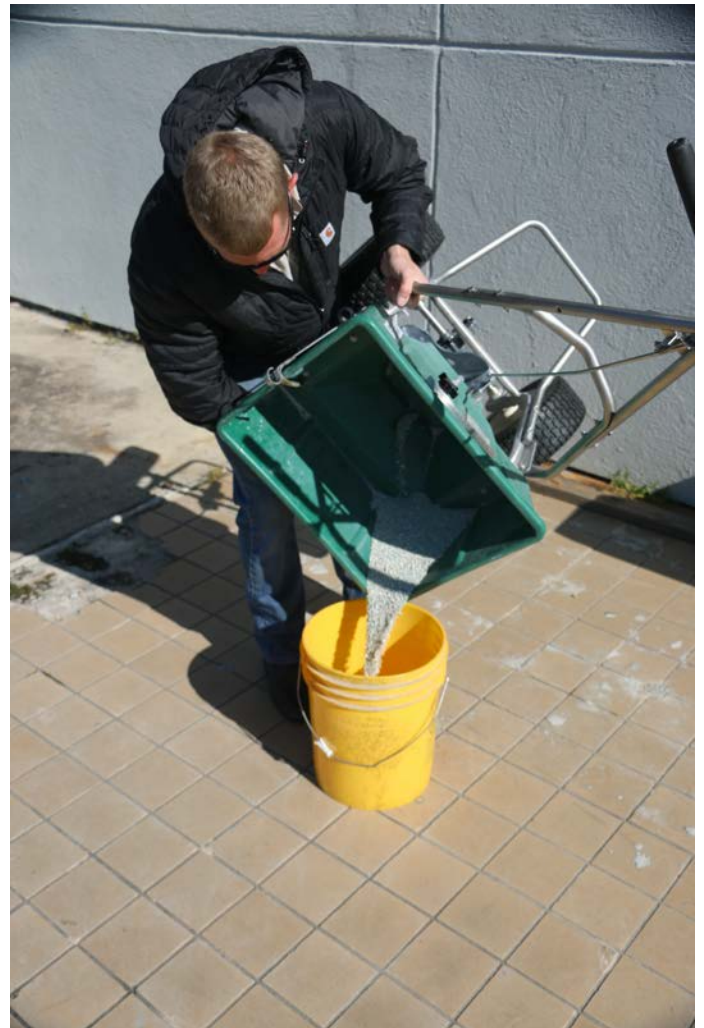
The material left in the spreader after walking the test strip is poured out to be weighed.
