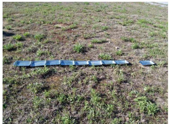
Pans labeled 0-9 placed in a straight line. A space is left between the "0" and "2" pans for the spreader wheel to pass through. Justin Ballew, ©2018, Clemson University
