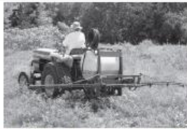
Top: Various size herbicide sprayers. Bottom: Fifty-gallon spray rig with a 15-foot boom is practical for sites larger than a half acre.
