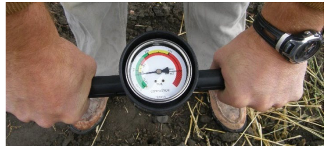
Image 1. Penetrometer used to measure soil resistance. Photo: Ross McKenzie.
