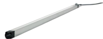
LI-191 R Line quantum sensor measures PAR (Photosynthetically Active Radiation) 2 days of data acquisition
