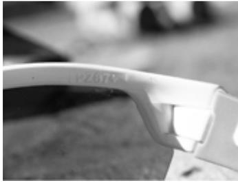
Figure 3: Impact-rated safety glasses that are safe to use with chainsaws should have the Z87+ lettering on the frame. In this example, the “P” in front of Z87+ indicates the manufacturer of the safety glasses. Photo Credit: Patrick Hiesl, Clemson University. In “How to Stay Safe Around Chainsaws,” Land-Grant Press by Clemson Extension, 2022.
