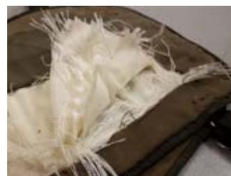
Figure 2: Cut-resistant material in chaps is typically embedded as multiple layers of woven material. Photo Credit: Patrick Hiesl, Clemson University. In "How to Stay Safe Around Chainsaws," Land-Grant Press by Clemson Extension, 2022.
