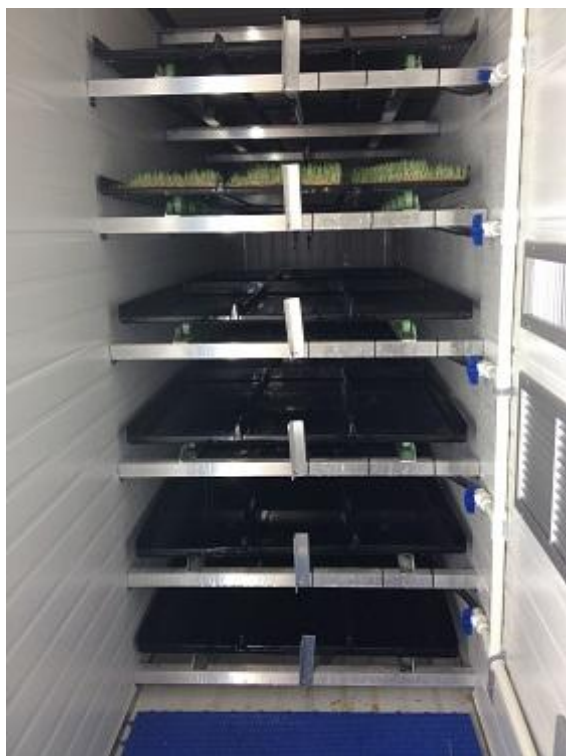
Figure 2. Fodder Machine, 9.8 ft. long X 5.7 ft. wide X 8.5 ft. tall, fully automatic growing chamber.
