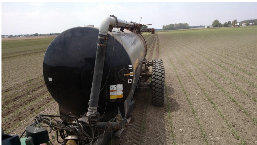
Figure 2. Narrow tires replaced the flotation tires on the manure tanker
