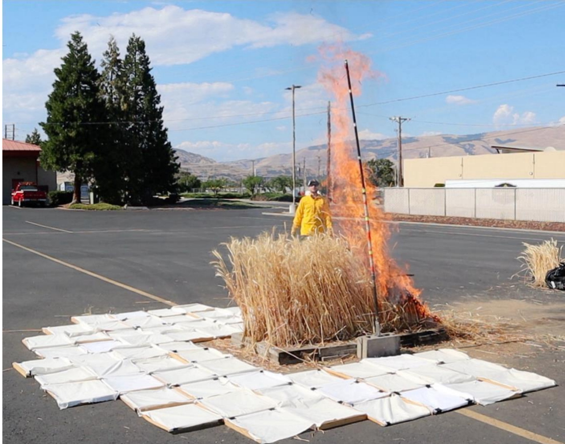
Figure 1. Experimental burn set up with dryland wheat and fire resistant fabric to quantify ember generation and flame height.
