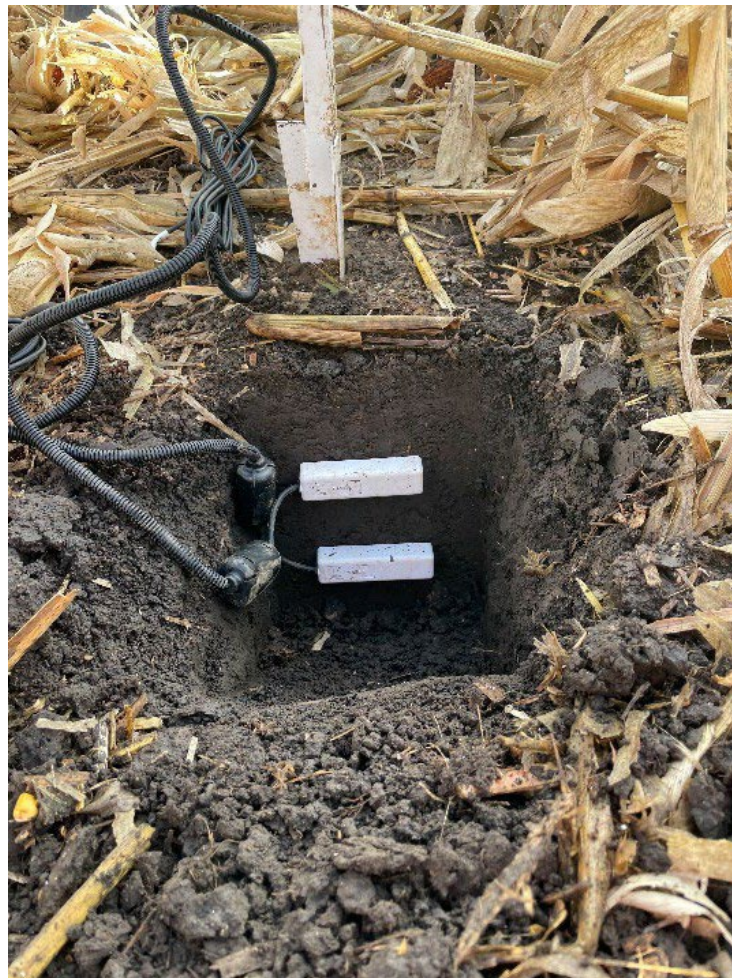
Figure 1. TEROS 11 sensors installed in the soil profile at 3- and 6-inch depth.
