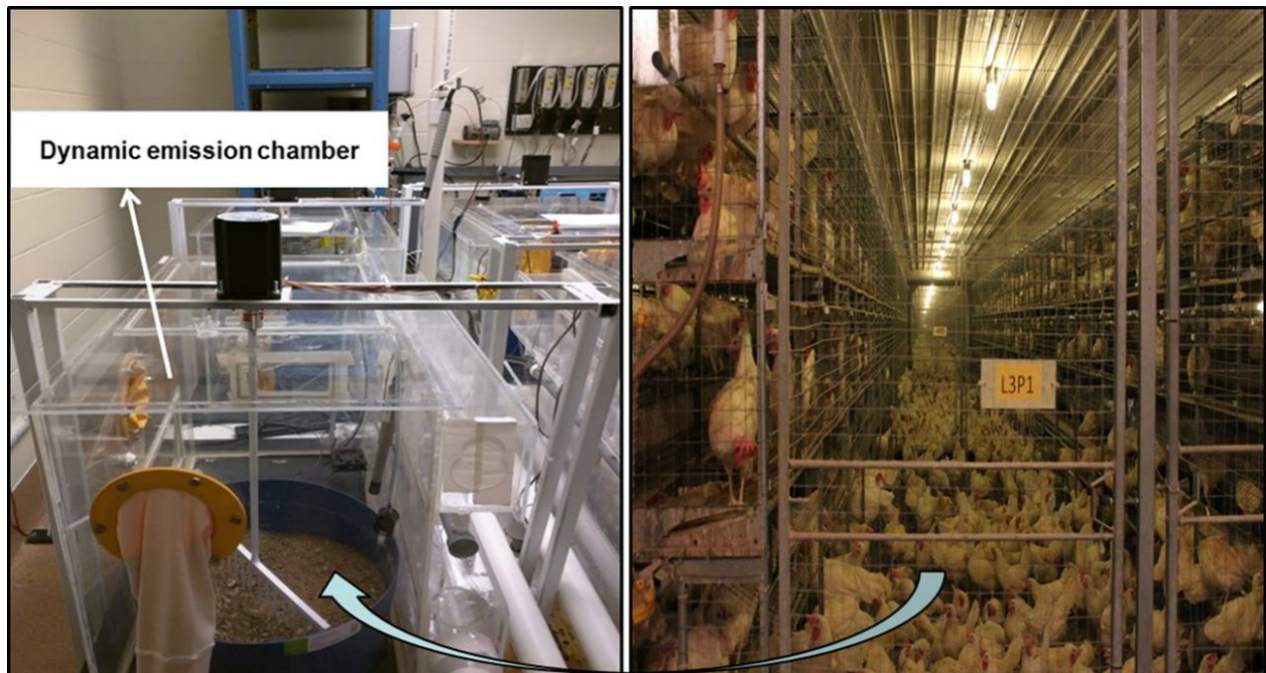
Figure 5. NH 3 mitigation test with dynamic emission chambers.
