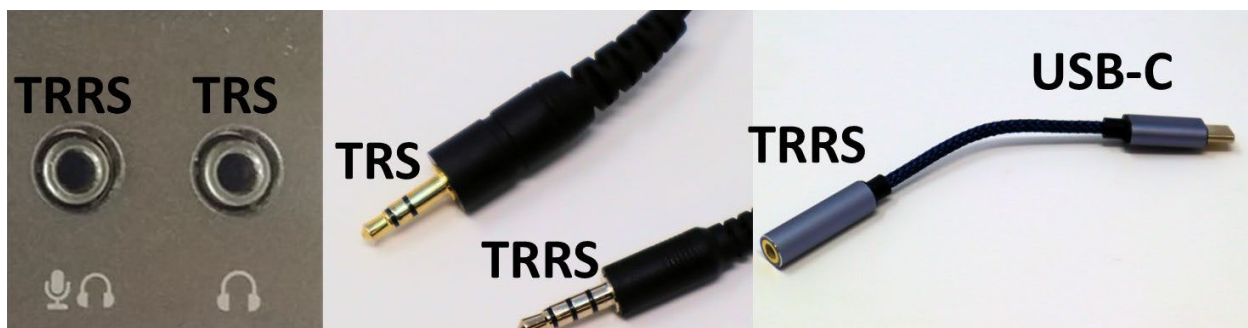
Figure 1. An example of a TRS, TRRS plugs and jacks, and a TRRS to USB-C adapter.
