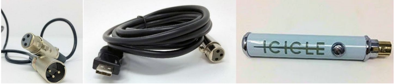
Figure 2. A microphone cable with XLR male and female connections along with two types of XLR to USB adapters.
