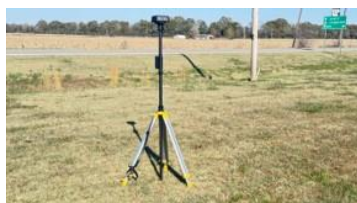
DJI RTK Base Station Gives the drone centimeter level accuracy
