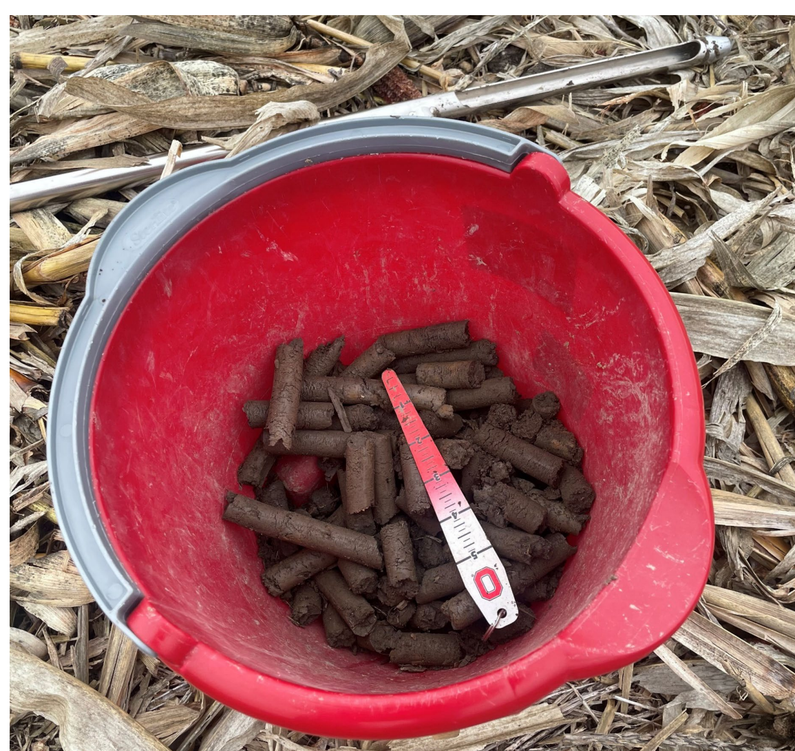
Image 1. Soil cores are collected from a corn field after harvest. This sample will be homogenized and submitted to a soil laboratory for analysis.
