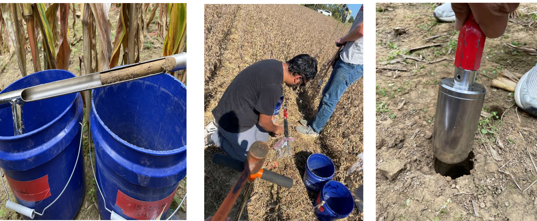
Fig.1 Soil sampling using the soil auger and soil core
