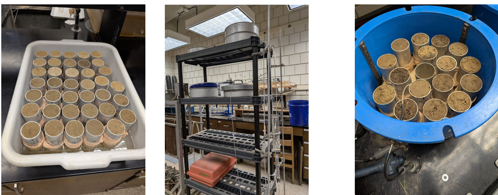
Fig.2 Processing of soil samples for soil moisture retention (a) soil saturation, (b) tension table (c) Pressure plate
