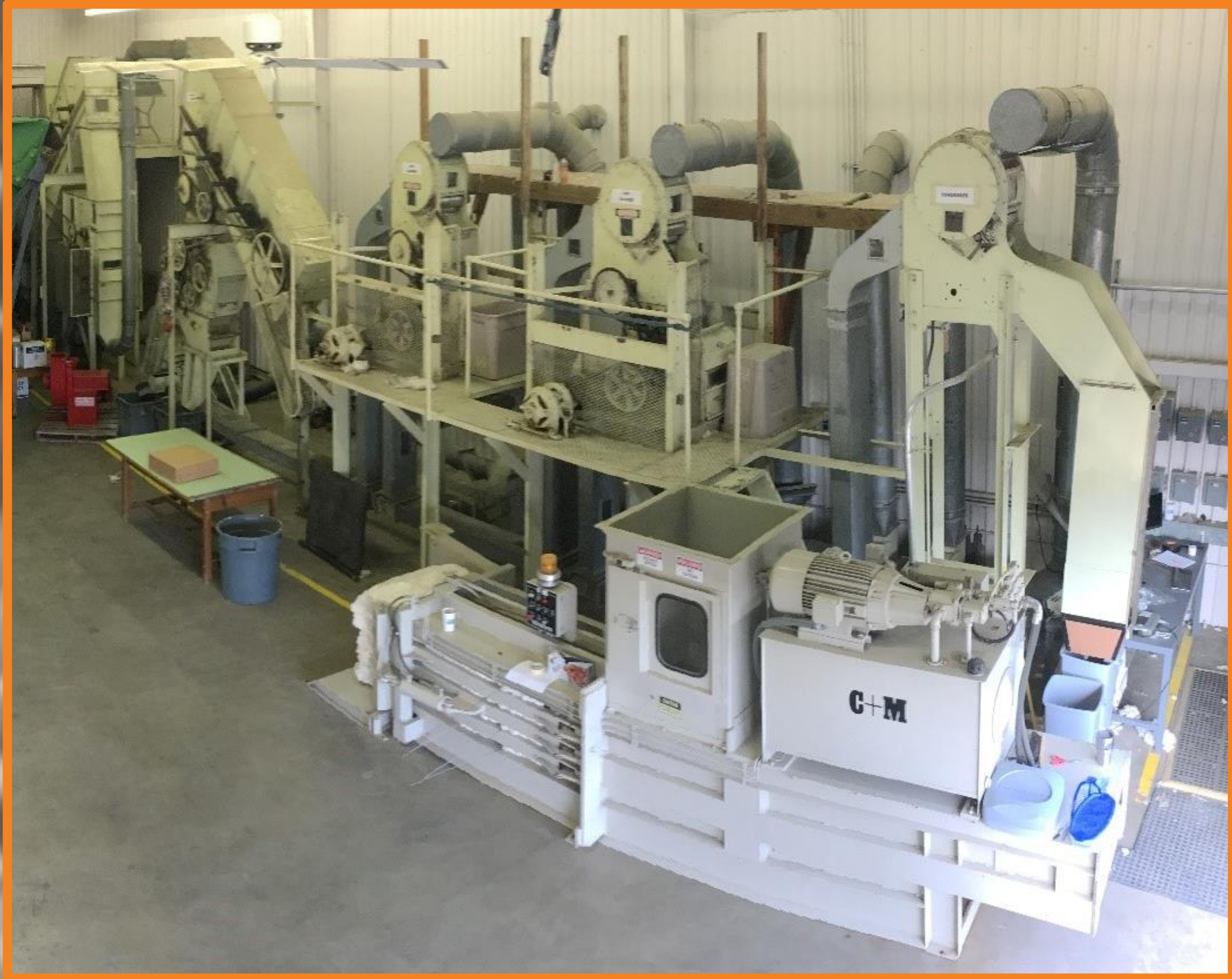
Figure 4: UT Cotton MicroGin located at the West Tennessee Research and Education Center in Jackson, TN. This is a 20-saw gin equipped with a stick machine, incline cleaners, and one lint cleaner.
