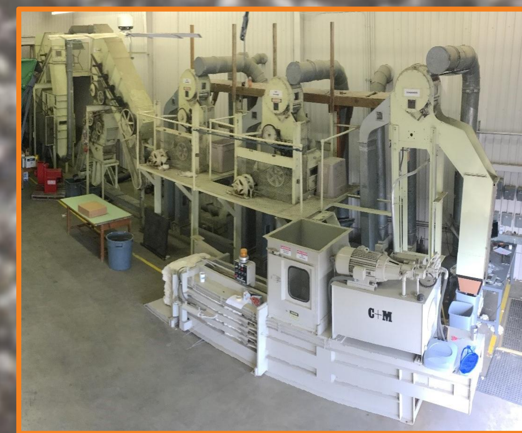
Fig. 4: UT Cotton MicroGin at the West Tennessee Research and Education Center in Jackson, TN, is a 20-saw gin equipped with a stick machine, incline cleaners, and one lint cleaner.
