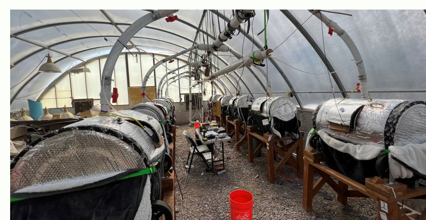
Heating blankets covering half of the reactors
