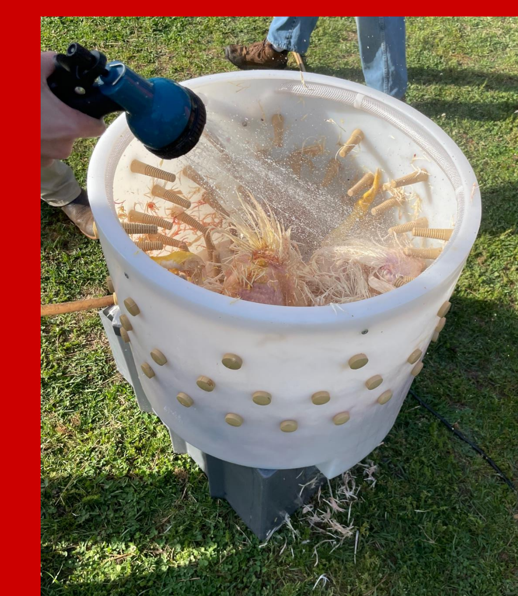
Step 3. The Plucker is a giant bin with rubber fingers that spins the birds to pull the feathers out. Water helps the feathers release and flow out of the plucker.
